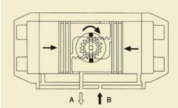
Air into Port A forces the pistons outwards, causing the pinion to turn counterclockwise while the air being exhausted from Port B.
